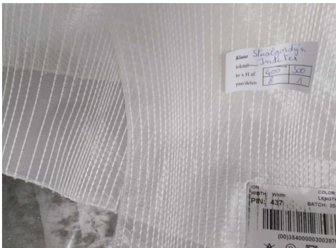
Distance d = 150\text{mm} (G150-mounting) Height [H] = 3200 mm Width covered surface = 4000 mm Pleated curtain : 180%, total width of the fabric = 7200mm
