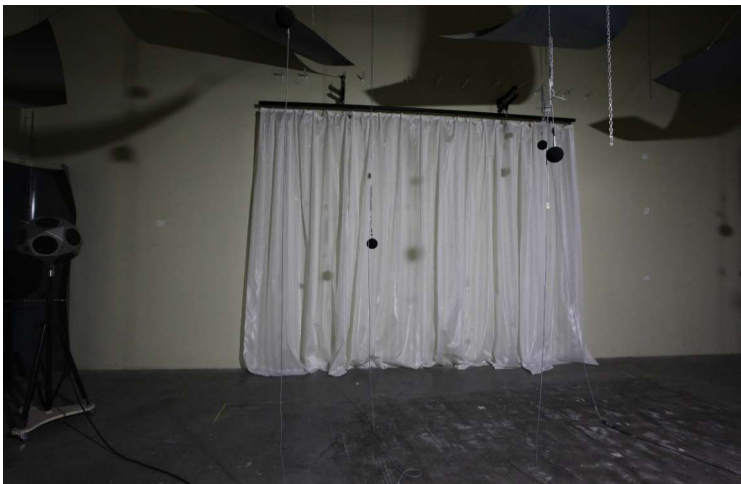
Distance d = 150\text{mm} (G150-mounting) Height [H] = 3200 mm Width covered surface = 4000 mm Pleated curtain : 180%, total width of the fabric = 7200mm
